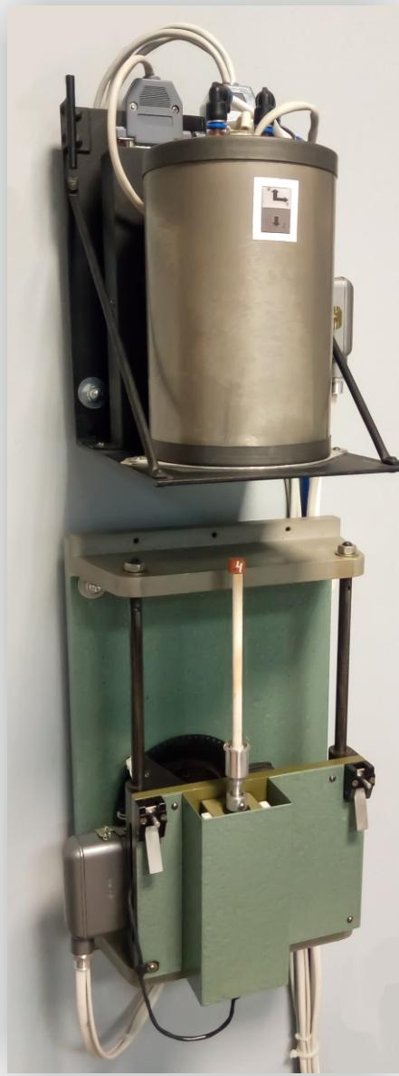
Orion is top-of-the-edge multifunctional device for rock magnetic, paleomagnetic, archeomagnetic and paleointensity studies. It combines a water-cooled furnace, controlled DC-field, and ultra sensitive magnetic sensors for full-vector measuring. The instrument is placed into a three-layer permalloy magnetic shield. The interface is a Windows-based user-friendly software with plain scripting language.
